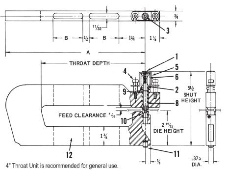
ALTERNATE ASSEMBLY FOR HOLE SIZE .125 AND UNDER
