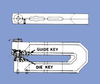
**KEYING ARRANGEMENT** FOR MODELS M1<sup>1</sup>/4, M1<sup>3</sup>/4, M2<sup>1</sup>/<sub>4</sub>, M2<sup>1</sup>/<sub>2</sub>, M3 & M4
