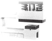
This unit has the capacity of punching holes in material up to <sup>3</sup>/<sub>4</sub>" thick.
